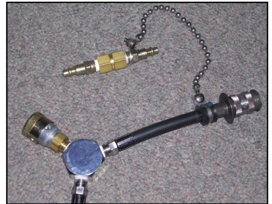
Photo-3: Low Pressure Manifold with EBSS
