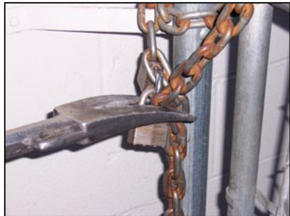
Photos 11 & 12: Using either the fork or pick of the halligan can be used when trying to defeat a pad-lock.
