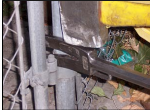
Photos 13 & 14: Attacking the hinge side of the gate is a quicker and easier method than trying to defeat a pad lock.
